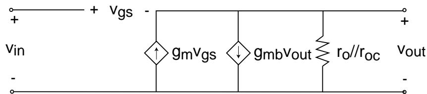
$$A_{vo} = \frac{g_m}{g_m + g_{mb} + \frac{1}{r_o//r_{oc}}} \simeq \frac{g_m}{g_m + g_{mb}} < 1$$
