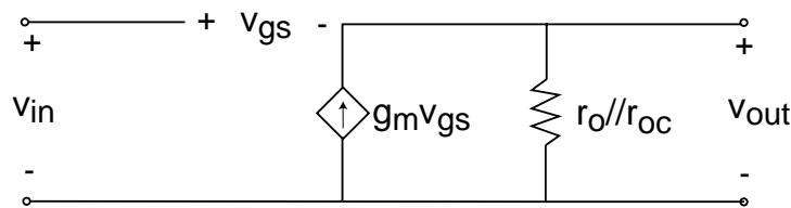
$$v_{in} = v_{gs} + v_{out}$$
