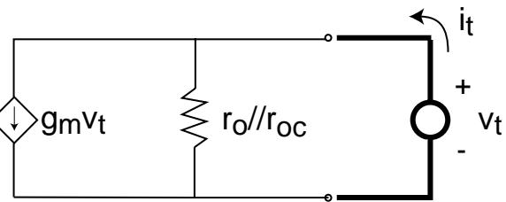
$$R_{out} = \frac{1}{g_m + \frac{1}{r_o // r_{oc}}} \simeq \frac{1}{g_m}$$
