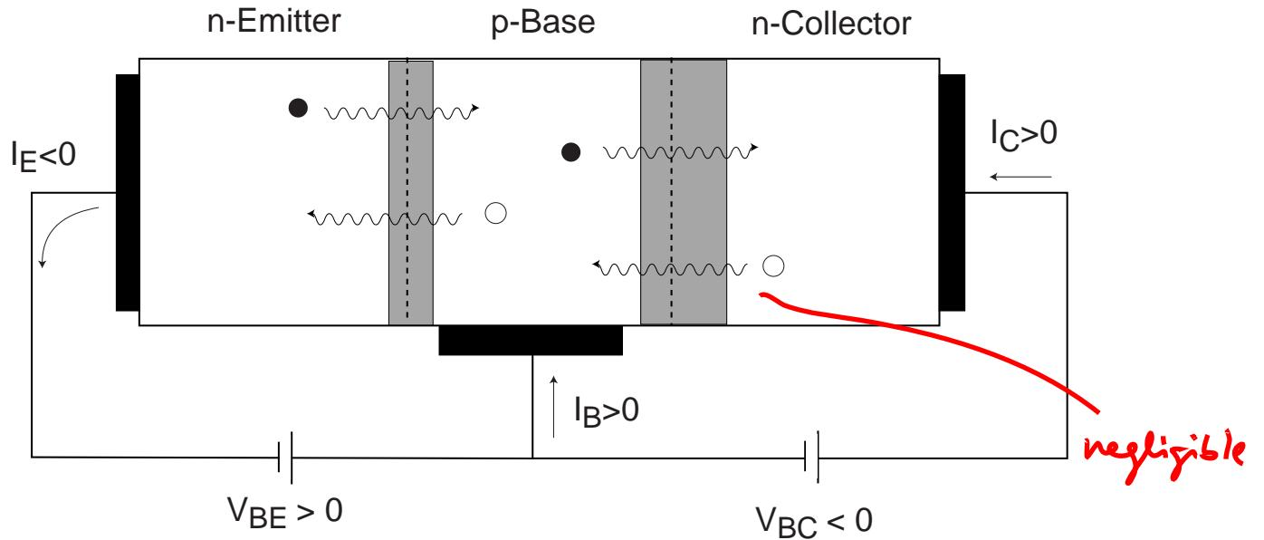
$V_{BE} > 0 \Rightarrow$  injection of electrons from E to B
