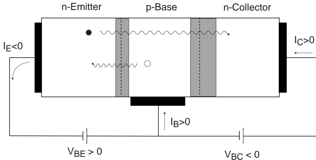
$I_C$ : electron injection from E to B and collection into C
