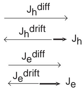
Current balance in SCR broken:
