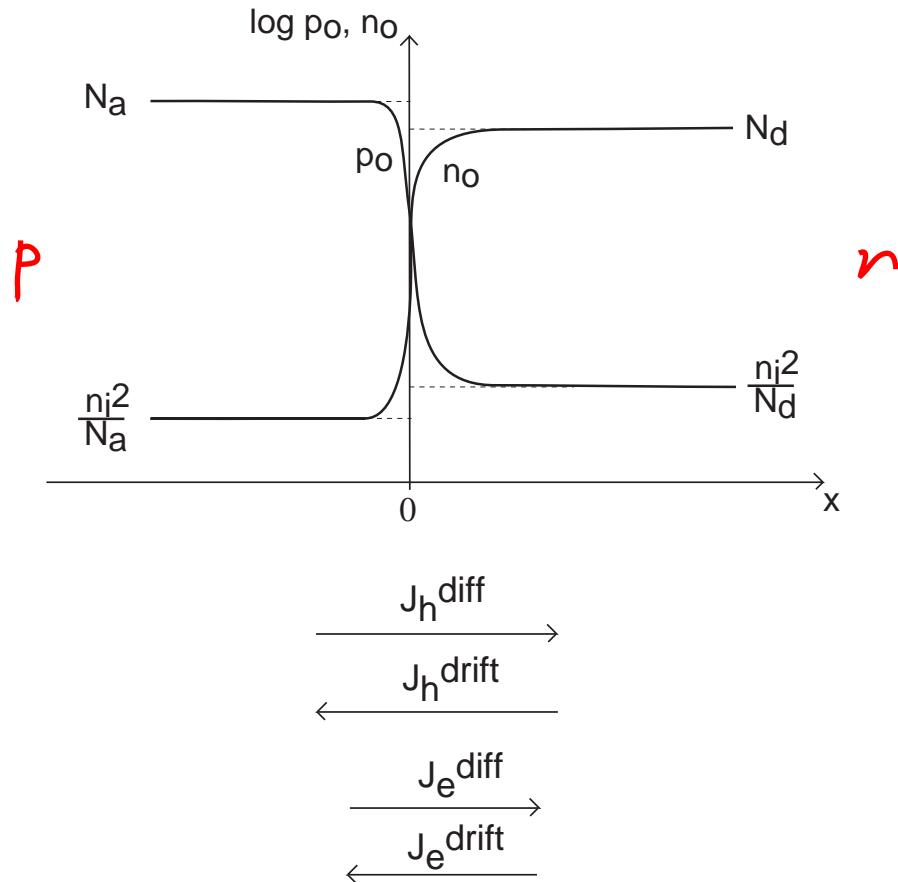
Inside SCR in thermal equilibrium: dynamic balance between drift and diffusion for electrons and holes.
