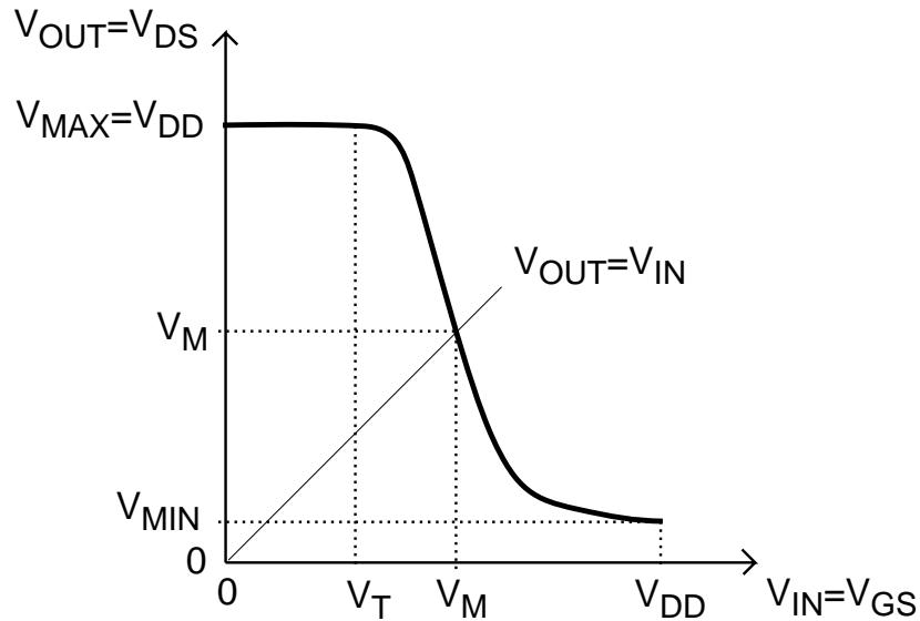
For  $V_{MAX}$ , transistor is cut-off,  $I_D = 0$ :
