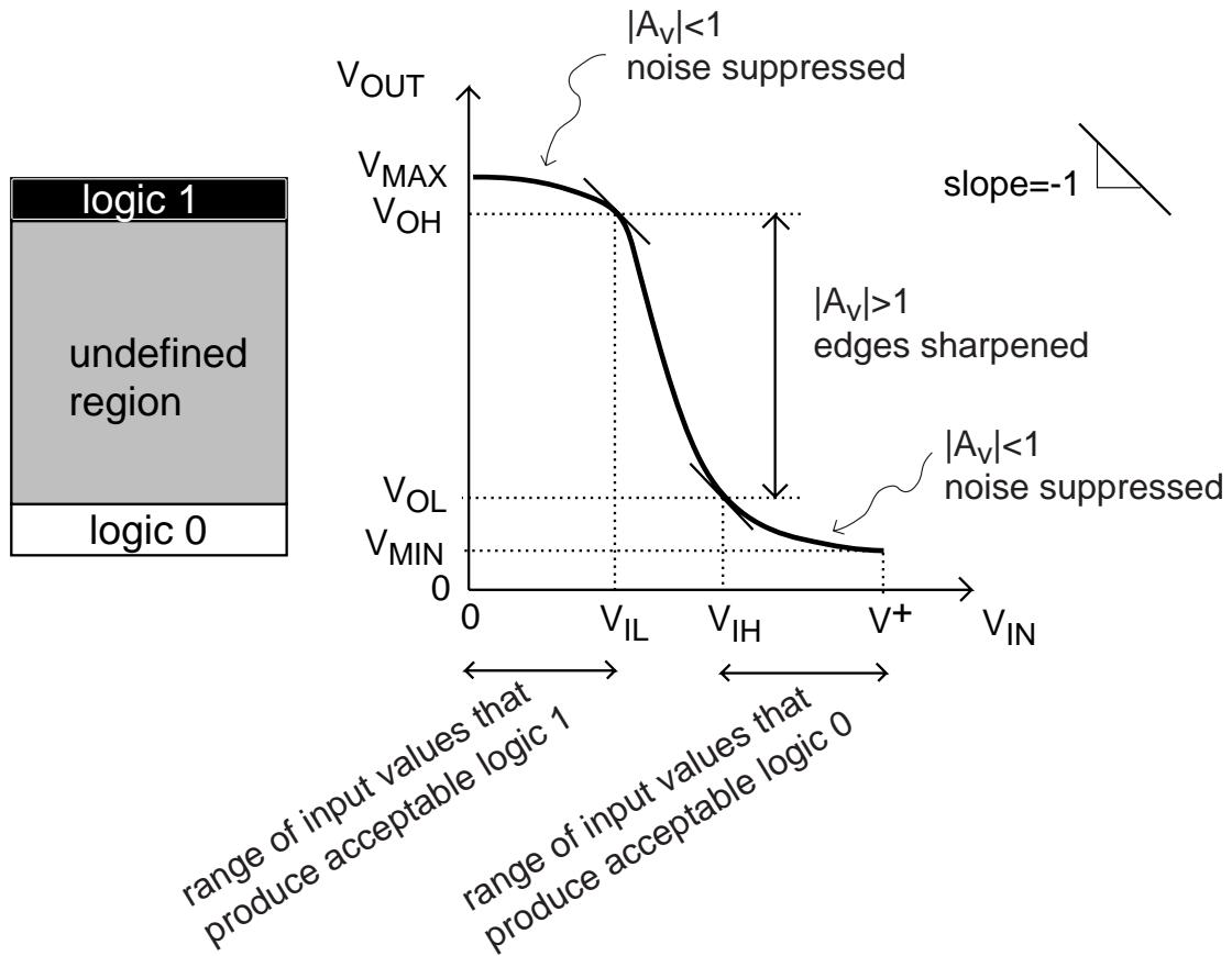
$V_{IL} \equiv$  smallest input voltage where slope=-1
