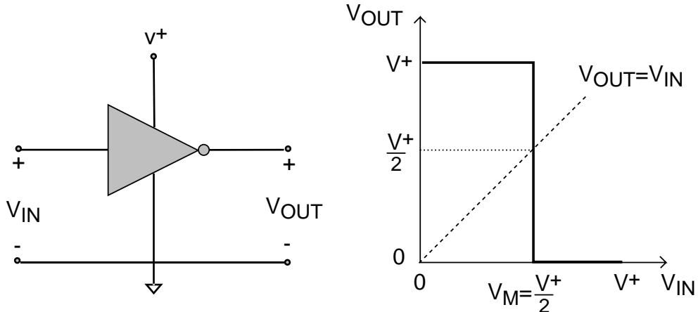
Define *switching point* or ***logic threshold***:
