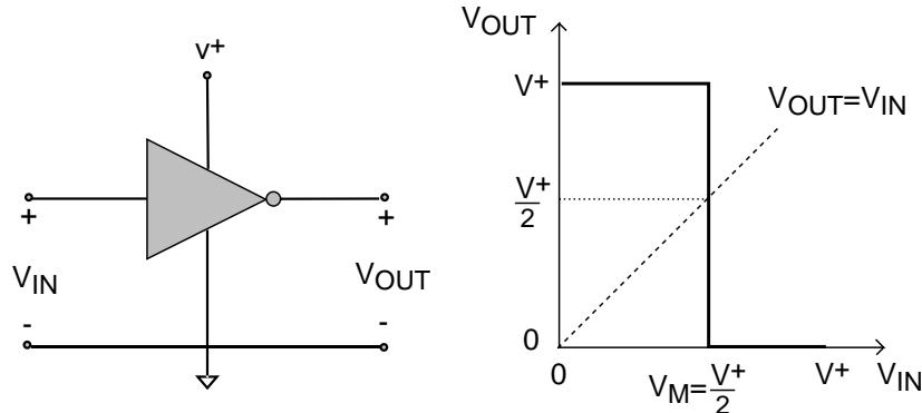
Ideal inverter returns well defined logical outputs (0 or  $V^+$ ) even in the presence of considerable noise in  $V_{IN}$  (from voltage spikes, crosstalk, etc.)
