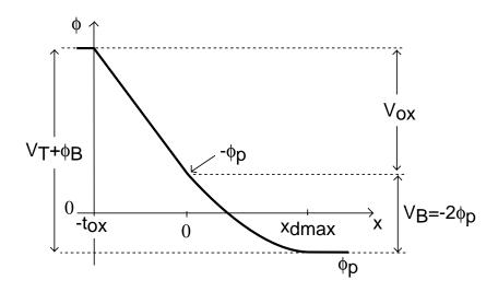
$$V_T + \phi_B = V_B(V_T) + V_{ox}(V_T) = -2\phi_p + \gamma\sqrt{-2\phi_p}$$
