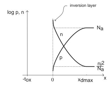
Electron concentration at Si/Si $O_2$  interface modulated by  $V_{GB} \Rightarrow V_{GB} \uparrow \rightarrow n(0) \uparrow \rightarrow |Q_n| \uparrow$  field-effect control of mobile charge! [essence of MOSFET]
