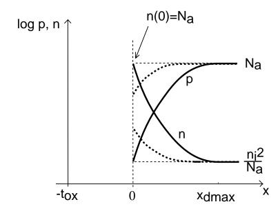
Let's compute the voltage (threshold voltage) that leads to  $n(0) = N_a$ .
