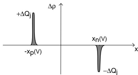
*Depletion capacitance per unit area (depletion approx.):*
