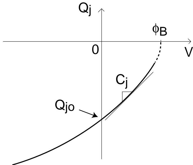
$C_j$  is slope of  $Q_j$  vs.  $V$  characteristics:
