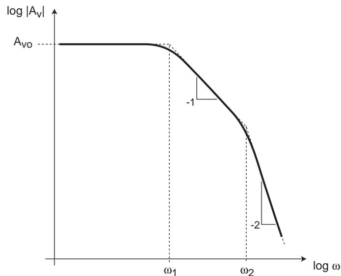
$$\frac{V_{out}}{V_s} = \frac{A_{vo}}{(1 + j\frac{\omega}{\omega_1})(1 + j\frac{\omega}{\omega_2})(1 + j\frac{\omega}{\omega_3})\dots}$$
