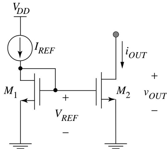
$$I_{OUT} \simeq \frac{1}{2} \left( \frac{W}{L} \right)_2 \mu C_{ox} (V_{REF} - V_T)^2$$
