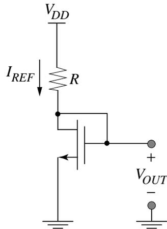
$$I_{REF} = \frac{V_{DD} - V_{OUT}}{R}$$
