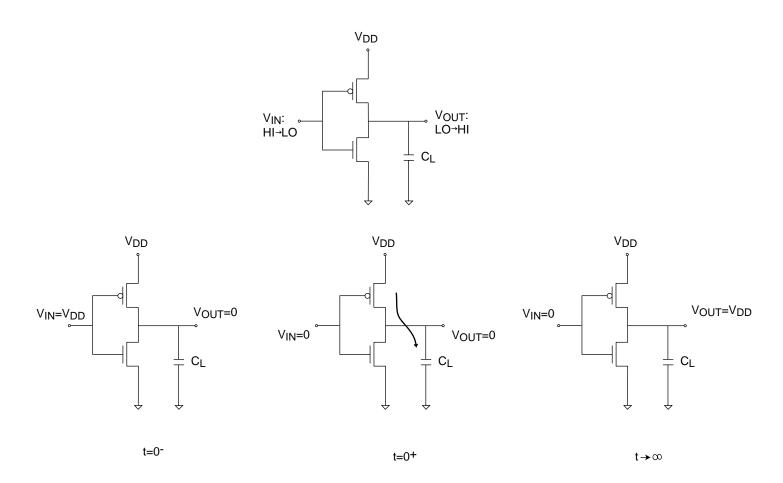
During early phases of charge, PMOS is saturated and NMOS is cut-off.
