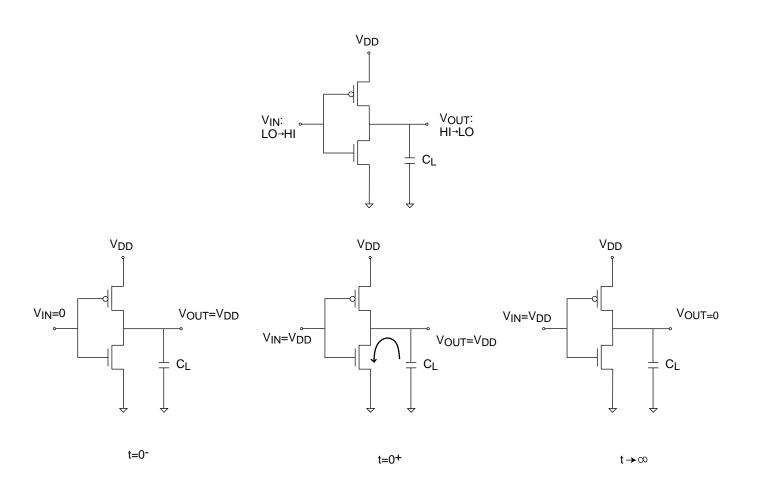
During early phases of discharge, NMOS is saturated and PMOS is cut-off.
