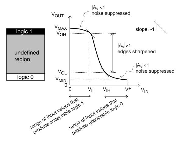
$V_{IL} \equiv \text{smallest input voltage where slope=-1}$
