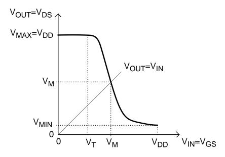
For  $V_{MAX}$ , transistor is cut-off,  $I_D = 0$ :
