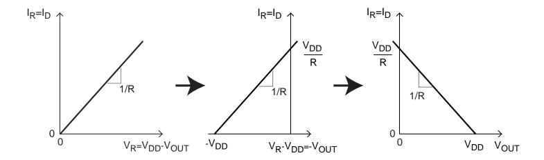
Overlap I-V characteristics of resistor pull-up on I-V characteristics of transistor:
