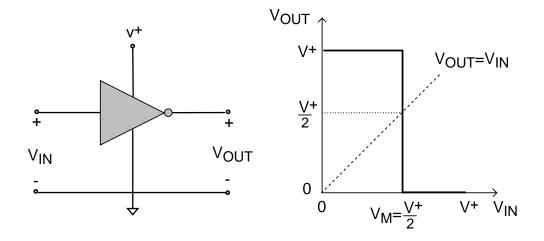
Define switching point or logic threshold:
