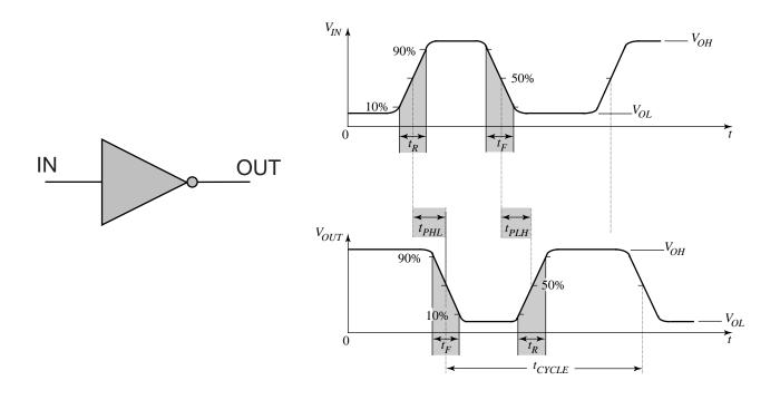
$t_R \equiv rise \ time \ between 10\% \ and 90\% \ of total swing$   $t_F \equiv fall \ time \ between 90\% \ and 10\% \ of total swing$   $t_{PHL} \equiv propagation \ delay \ from \ high-to-low \ between 50\% \ points$
