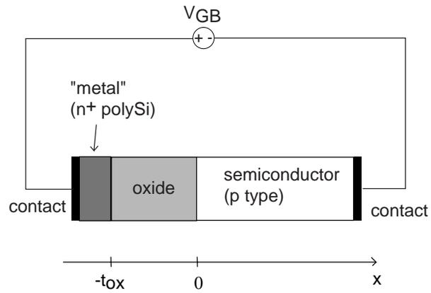
The oxide thickness is  $t_{ox} = 50 \text{ nm}$  and the doping level in the substrate is  $N_a = 10^{16} \text{ cm}^{-3}$ .
