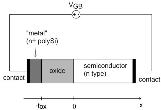
The doping level in the substrate (or body) is  $N_D = 10^{17} \text{ cm}^{-3}$ . The doping level in the gate is  $N_D^+ = 10^{20} \text{ cm}^{-3}$ .
