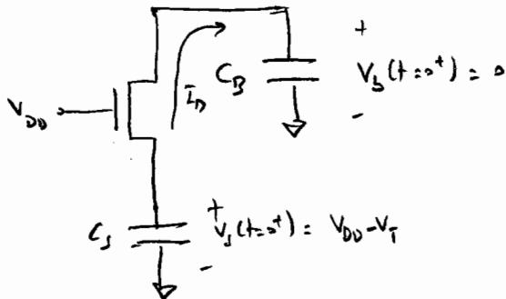
This is a situation identical to that of 4f. The transistor is therefore at the boundary between the linear and the saturation regimes.
