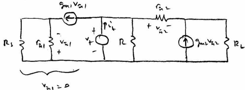
$$i_t = \frac{V_t}{R} + \frac{v_{a2}}{r_{a2}}$$
