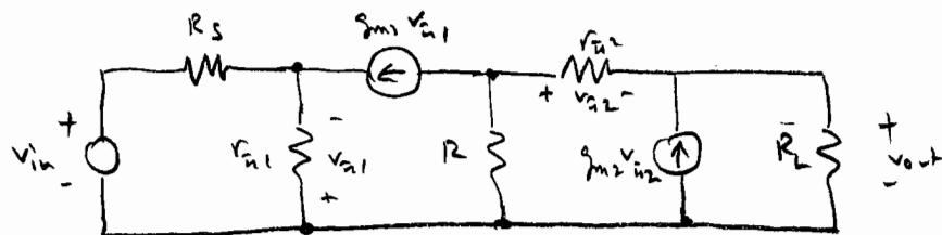
We relate  $v_{in}$  to  $v_{21}$ :
