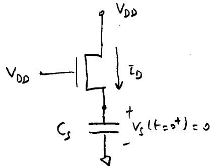
The source is at 0 while the gate and drain are at  $V_{DD}$ . Then, the transistor is in saturation.
