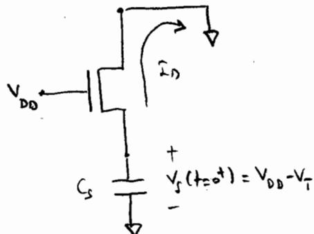
Notice that in this case, current will bleed off upwards through the MOSFET into ground. The top terminal is therefore the source and the bottom one is the drain. Then
