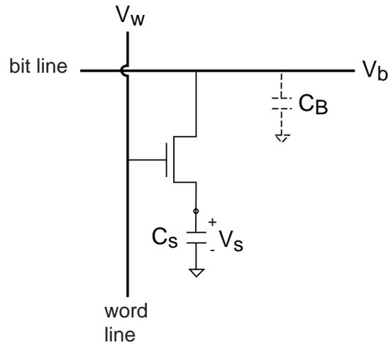
In this DRAM cell, the information is stored in the form of charge in the capacitor  $C_s$ . If the voltage across the capacitor  $V_s$  is HI, then a "1" is stored. If  $V_s$  is LO, a "0" is stored.
