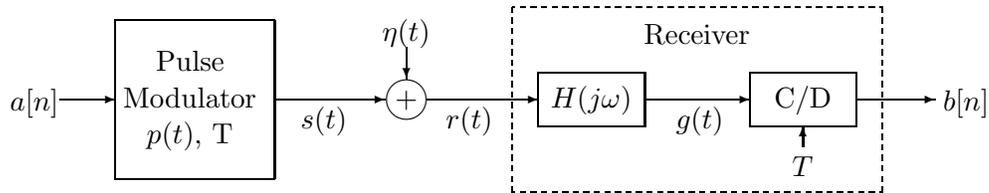
Figure 7-1: PAM system with receiver filter  $h(t)$
