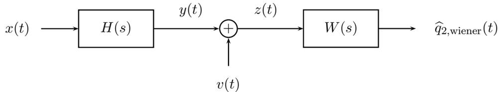
Figure 6-2: Noncausal Wiener filter based system
