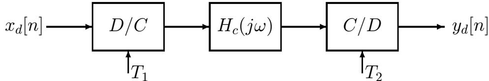
We are assuming we have an ideal D/C converter. The output of the D/C converter,  $x_c(t)$ , is always bandlimited to  $|\omega| = \frac{\pi}{T}$ . As a result, the input to the C/D is always appropriately bandlimited, and no aliasing occurs.
