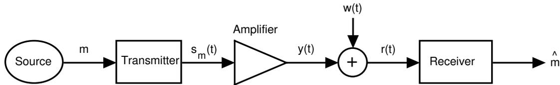
Figure 6-1: Baseband model for a communication system with in-line amplification.
