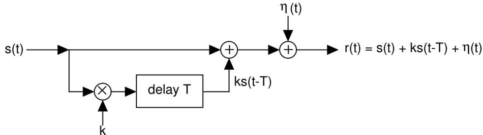
Figure 3-1: Channel model for a wireless communication system.
