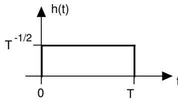
Figure 6-4: Impulse response  $h(t)$  of the receiver filter.
