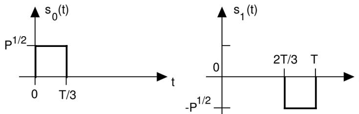
Figure 6-2: Transmitter waveforms  $s_0(t)$  and  $s_1(t)$ ;  $P$  is the transmitter's peak instantaneous power.
