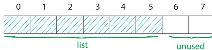
Figure 2: Resizable Arrays
