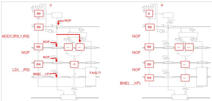
E. **Scenario 5:** (show 3 cycles of snapshot) Show what happens when an interrupt occurs when the Beta is fetching the SUB instruction. Assume the hardware sets PC<sup>IF</sup> to 0 when taking an interrupt.
