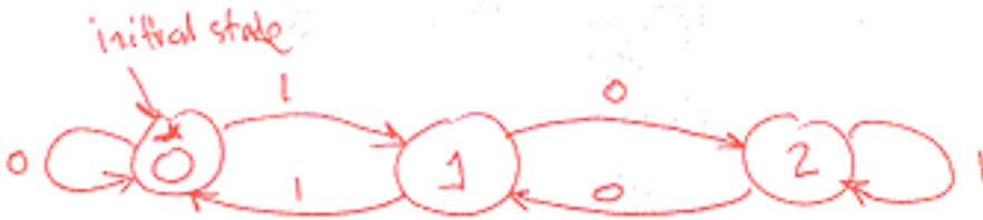
B. ★ Construct a truth table for the FSM logic. Inputs include the state bits and the next bit of the number; outputs include the next state bits and the control for the light.
