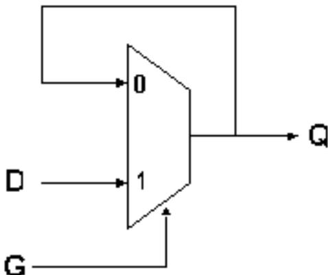
Recall that the MUX selects the Q output when  $G=0$ , and the D input when  $G=1$ . The plan is that when  $G=1$ , the Q output will follow D after a short delay; when  $G=0$ , the current Q output will be "latched" via the feedback path. In this problem we explore assumptions necessary to construct an informal proof that the latch behaves as proposed. Assume, in each of the following, that the MUX is a well-behaved lenient combinational device with a propagation delay of  $t_{pd}$ .
