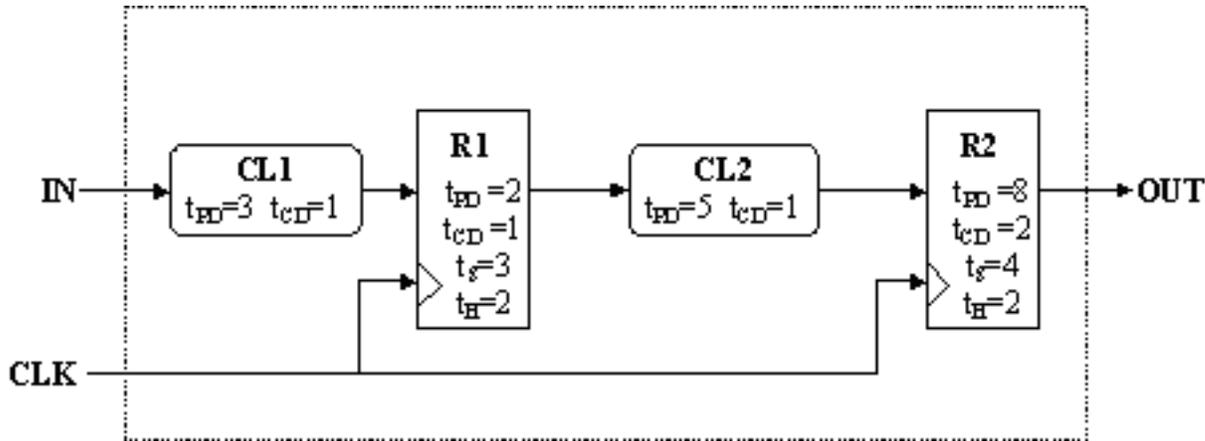
The components labeled CL1 and CL2 are combinational; R1 and R2 are edge-triggered flip flops. Timing parameters for each component are as noted.
