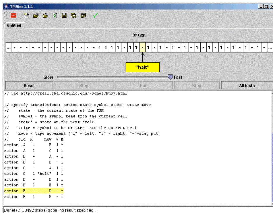
The TM display consists of the following parts:
