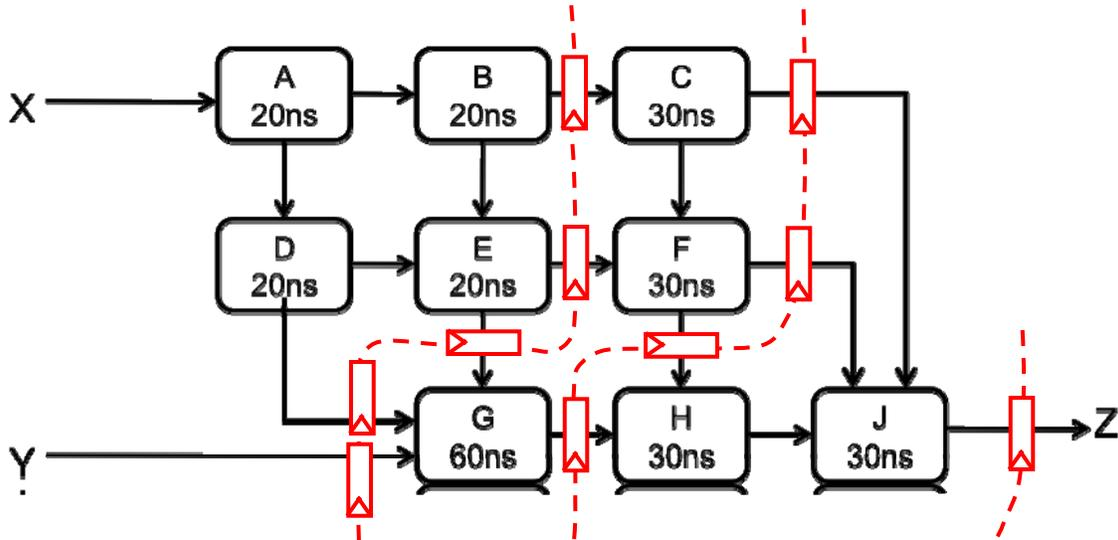
Although you don't know the function of each of the component modules, they are each combinational and marked with their respective propagation delays. You have been hired to analyze and improve the performance of this device.
