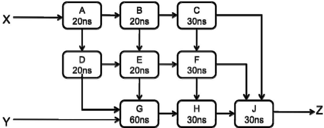
Although you don't know the function of each of the component modules, they are each combinational and marked with their respective propagation delays. You have been hired to analyze and improve the performance of this device.
