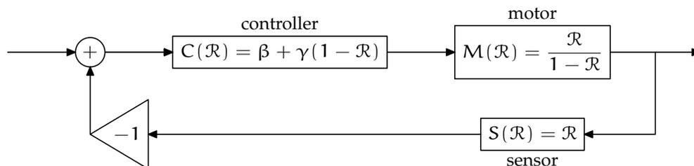
Let  $F(\mathcal{R})$  be the functional for the entire feedback system. Its numerator is the forward path  $C(\mathcal{R})M(\mathcal{R})$ . Its denominator is  $1 - L(\mathcal{R})$ , where  $L(\mathcal{R})$  is the loop functional or **loop gain** that results from going once around the feedback loop. Here the loop functional is
