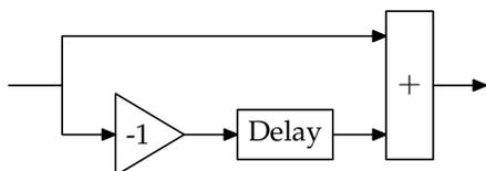
where the gain of  $-1$  produces the subtraction.
