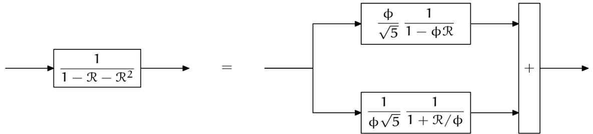
where, to make the diagram easier to parse, system functionals stand for the first- and second-order systems that they represent.
