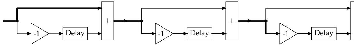
Besides the two delays, each path accumulates two gains of  $-1$ , making a gain of 1. So the sum of the three paths is a gain of 3 and a double delay.
