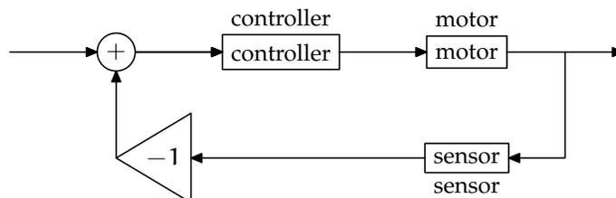
A real sensor cannot respond instantaneously, so assume the next-best situation, that the sensor includes one unit of delay. Then the sensor's output gets subtracted from the desired angle to get the error signal, which is used
