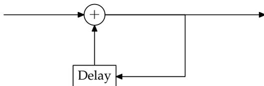
Now combine the visual virtues of block diagrams with the compactness and symbolic virtues of operators by using  $\mathcal{R}$  instead of 'Delay'. The operator block diagram is
