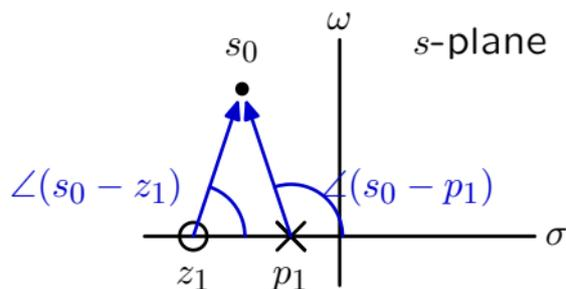
The angle of  $K$  can be 0 or  $\pi$  for systems described by linear differential equations with constant, real-valued coefficients.
