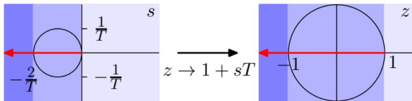
DT stability: CT pole must be inside circle of radius  $\frac{1}{T}$  at  $s = -\frac{1}{T}$ .
