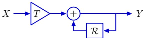
Backward Euler: substitute equivalent system for all integrators.
