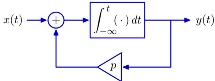
Delays in DT are replaced by integrators in CT.
