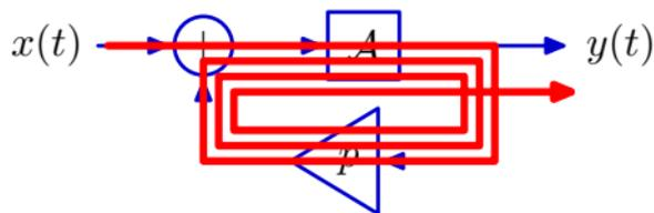
$$\begin{aligned}y(t) &= (\mathcal{A} + p\mathcal{A}^2 + p^2\mathcal{A}^3 + p^3\mathcal{A}^4 + \dots) \delta(t) \\ &= (1 + pt + \frac{1}{2}p^2t^2 + \frac{1}{6}p^3t^3 + \dots) u(t) = e^{pt}u(t)\end{aligned}$$
