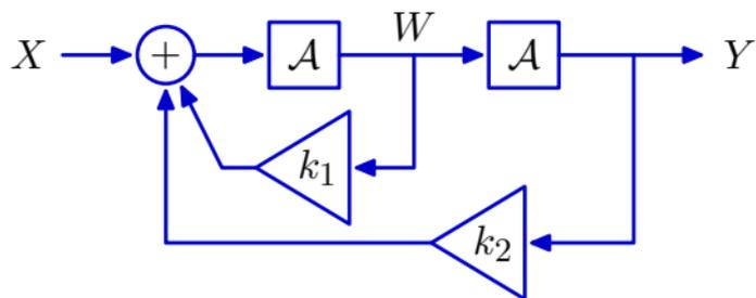
$$\begin{aligned} W &= \mathcal{A}(X + k_1W + k_2Y) & Y &= \mathcal{A}^2X + k_1\mathcal{A}Y + k_2\mathcal{A}^2Y \\ Y &= \mathcal{A}W & (1 - k_1\mathcal{A} - k_2\mathcal{A}^2)Y &= \mathcal{A}^2X \end{aligned}$$
