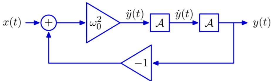
$$\frac{Y}{X} = \frac{\omega_0^2 \mathcal{A}^2}{1 + \omega_0^2 \mathcal{A}^2} = \omega_0^2 \mathcal{A}^2 - \omega_0^4 \mathcal{A}^4 + \omega_0^6 \mathcal{A}^6 - + \dots$$
