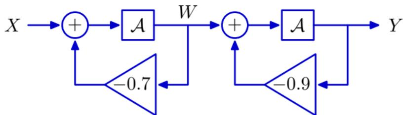
$$\begin{aligned} W &= \mathcal{A}(X - 0.7W) & (1 + 0.7\mathcal{A})W &= \mathcal{A}X & (1 + 0.7\mathcal{A})(1 + 0.9\mathcal{A})Y &= \mathcal{A}^2X \\ Y &= \mathcal{A}(W - 0.9Y) & (1 + 0.9\mathcal{A})Y &= \mathcal{A}W & (1 + 1.6\mathcal{A} + 0.63\mathcal{A}^2)Y &= \mathcal{A}^2X \end{aligned}$$
