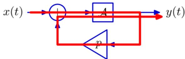
$$\begin{aligned}y(t) &= (\mathcal{A} + p\mathcal{A}^2 + p^2\mathcal{A}^3 + p^3\mathcal{A}^4 + \dots) \delta(t) \\ &= (1 + pt + \frac{1}{2}p^2t^2 + \frac{1}{6}p^3t^3 + \dots) u(t)\end{aligned}$$
