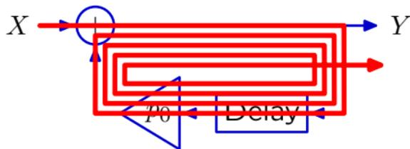
$$\begin{aligned}y[n] &= (1 + p\mathcal{R} + p^2\mathcal{R}^2 + p^3\mathcal{R}^3 + p^4\mathcal{R}^4 + \dots) \delta[n] \\ &= \delta[n] + p\delta[n-1] + p^2\delta[n-2] + p^3\delta[n-3] + p^4\delta[n-4] + \dots\end{aligned}$$
