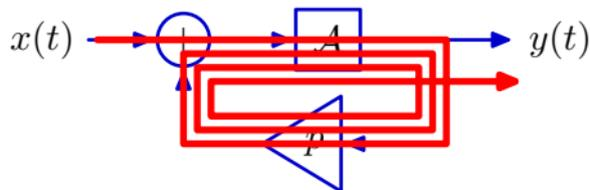
$$\begin{aligned}y(t) &= (\mathcal{A} + p\mathcal{A}^2 + p^2\mathcal{A}^3 + p^3\mathcal{A}^4 + \dots) \delta(t) \\ &= (1 + pt + \frac{1}{2}p^2t^2 + \frac{1}{6}p^3t^3 + \dots) u(t) = e^{pt}u(t)\end{aligned}$$
