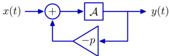
$$\begin{aligned}y(t) &= (\mathcal{A} - p\mathcal{A}^2 + p^2\mathcal{A}^3 - p^3\mathcal{A}^4 + \dots) \delta(t) \\ &= (1 - pt + \frac{1}{2}p^2t^2 - \frac{1}{6}p^3t^3 + \dots) u(t)\end{aligned}$$
