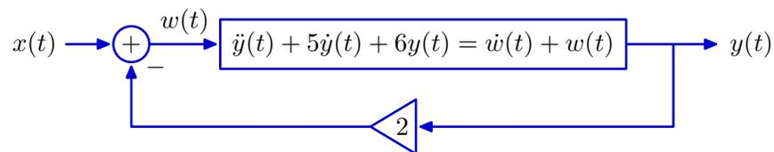
Determine a differential equation that relates the input  $x(t)$  and output  $y(t)$  of the closed loop system. Your answer should **NOT** depend on  $w(t)$  or any of its derivatives.
