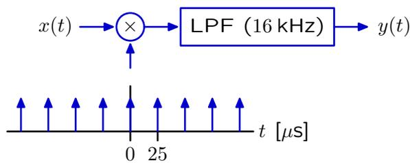
The plot below shows the Fourier transform  $Y$  of the output signal, for frequencies between 0 and 20 kHz. Write the number of the harmonic of  $x(t)$  that produced each component of  $Y$  in the box above that component. If none of 1-7 could have produced this frequency, enter **X**.
