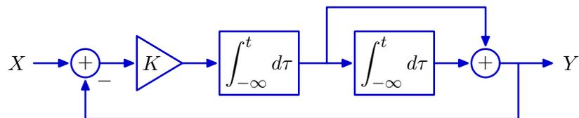
**Part a.** [10 points] Determine the system function  $H(s) = \frac{Y(s)}{X(s)}$  as a function of  $K$ .
