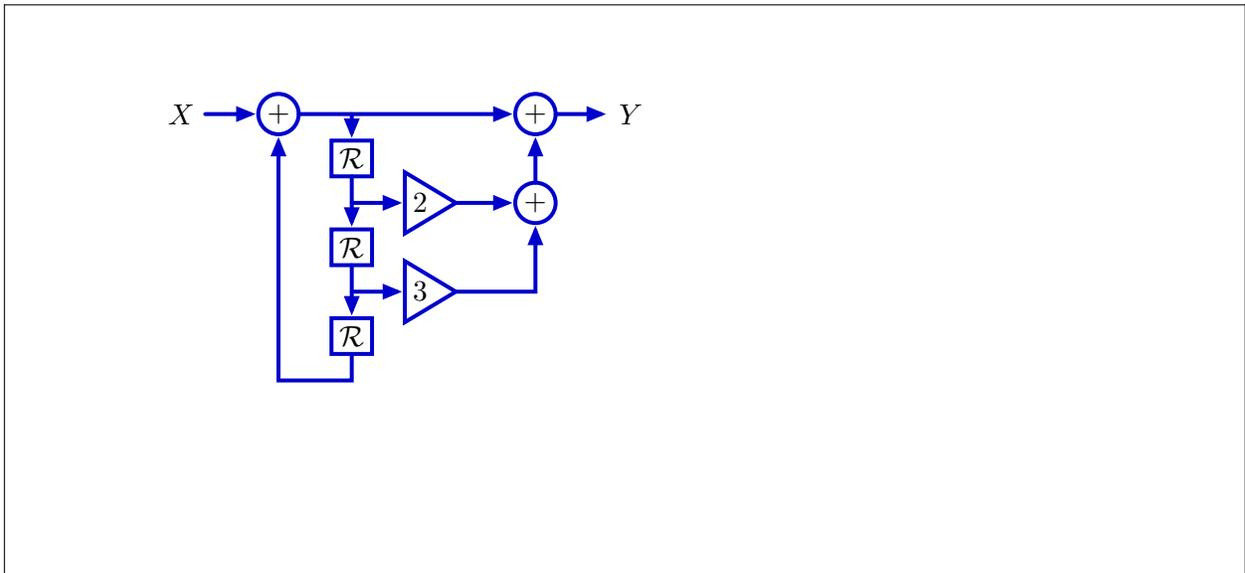
Derive the difference equation. The periodicity of 3 suggests that  $y[n]$  depends on  $y[n - 3]$ . To get the correct numbers, just delay the input and weight the delays appropriately. The resulting difference equation is
