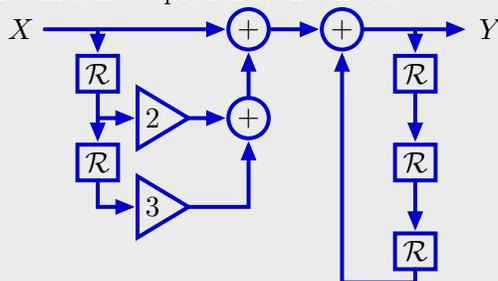
We can “reuse” 2 delays by commuting the left and right parts of this network, which gives the answer above.
