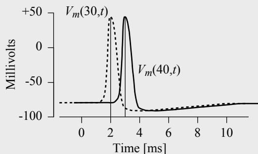
**Part b.** Sketch the dependence of  $V_m$  on  $z$  at time  $t = 0$  ms (i.e.,  $V_m(z, 0)$ ).
