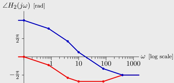
$H_2$  could also be multiplied by  $-1$  without having any effect on the magnitude function. Multiplying by  $-1$  would shift the phase curves up or down by  $\pi$ .
