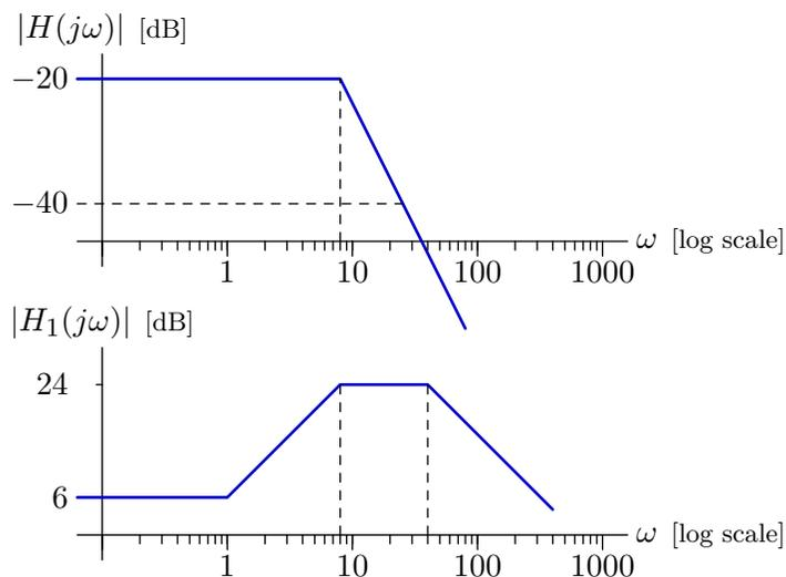
$H_1$  and  $H_2$  have to be stable as well as causal because we're talking about their frequency responses, and  $H$  has to be causal because  $H_1$  and  $H_2$  are. This implies that all poles must be in the left half-plane.
