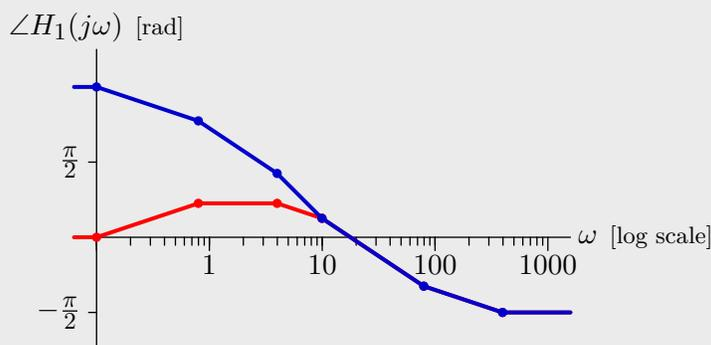
$H_1$  could also be multiplied by  $-1$  without having any effect on the magnitude function. Multiplying by  $-1$  would shift the phase curves up or down by  $\pi$ .
