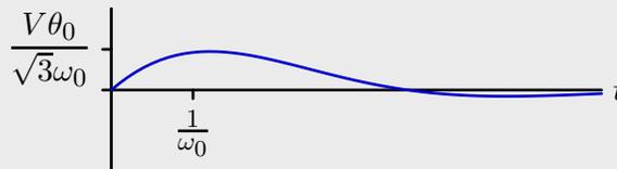
Increasing  $Q$  would reduce the overshoot but slow the response. We could compensate for the slowing of the response by increasing  $\omega_0$ .
