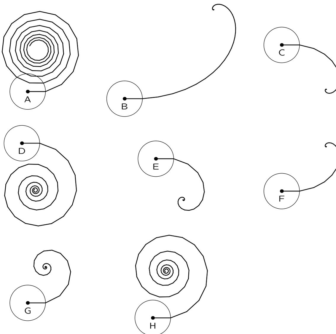
The first two terms in the series representation of  $S$  are 1 and  $0.8 + 0.2j$ . All of the curves start with a horizontal line to the right that stops at the intersection with the unit circle. Thus all of the curves correctly represent the first term. The second term should have a length that is somewhat shorter than 1 and an angle of  $\tan^{-1}(0.25)$ . We can immediately
