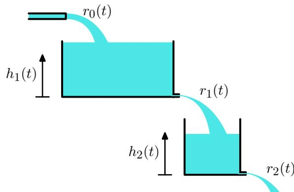
The rate of flow out of each tank is proportional to the height of the water in that tank:  $r_1(t) = k_1 h_1(t)$  and  $r_2(t) = k_2 h_2(t)$ , where  $k_1$  and  $k_2$  are each  $0.2 \text{ m}^2/\text{second}$ . Both tanks have heights of 1 m. The cross-sectional area of tank 1 is  $A_1 = 4 \text{ m}^2$  and that of the second tank is  $A_2 = 2 \text{ m}^2$ . At time  $t = 0$ , both tanks are empty.
