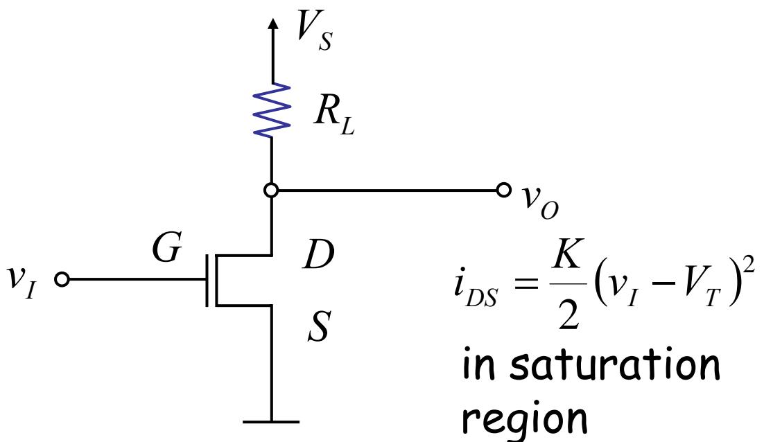
To ensure the MOSFET operates as a VCCS, we must operate it in its saturation region only. To do so, we promise to adhere to the “saturation discipline”
