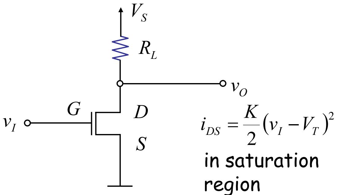
To ensure the MOSFET operates as a VCCS, we must operate it in its saturation region only. We promise to adhere to the "saturation discipline."
