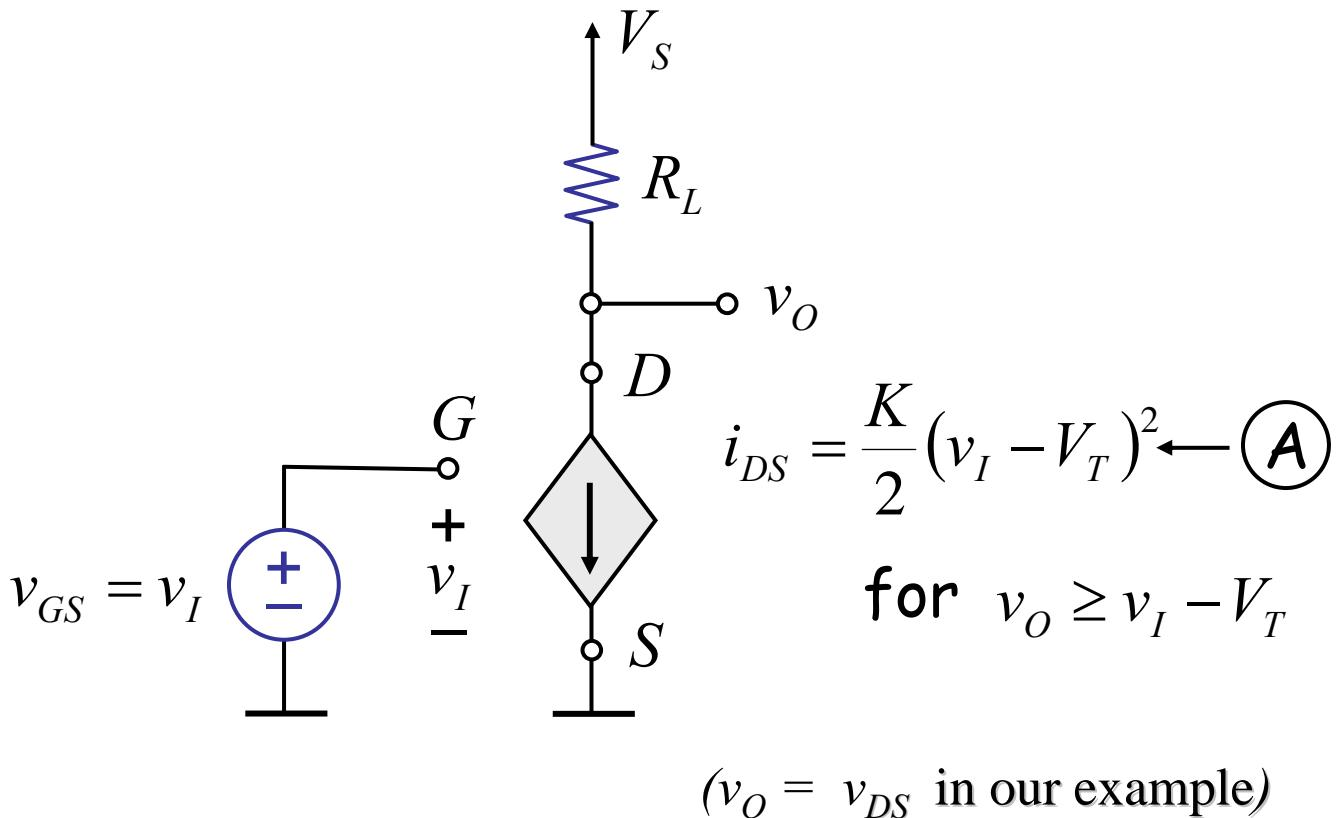
① Analytical method:  $v_O$  vs  $v_I$
