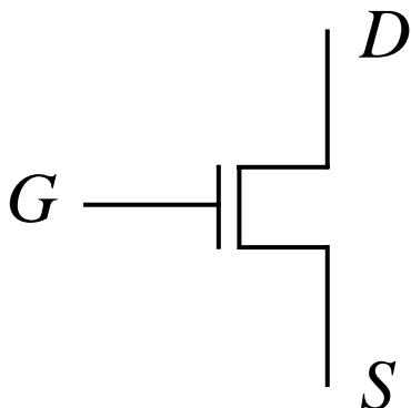
on when  $v_{GS} \geq V_{TN}$
