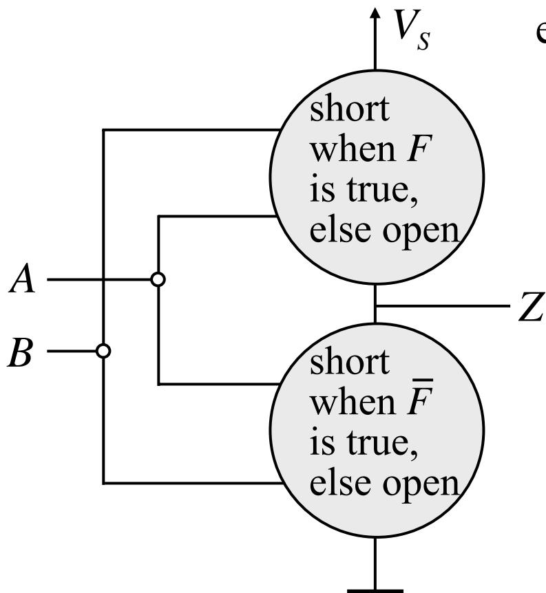
$$\text{e.g. } F = \overline{A \cdot B} = \overline{A} + \overline{B}$$
