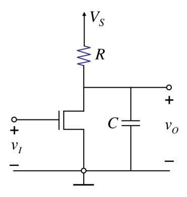
C: wiring capacitance and  $C_{GS}$  of following gate
