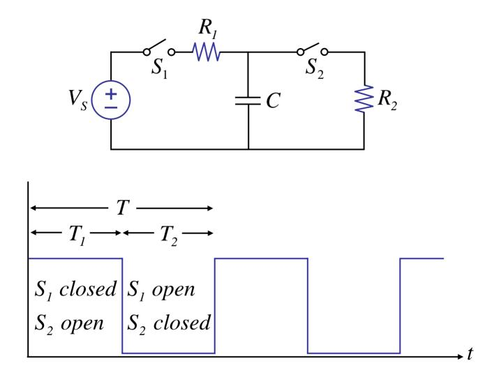
Find energy dissipated in each cycle. Find average power  $\overline{P}$ .
