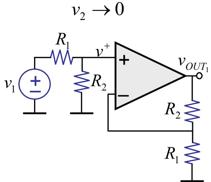
$$\begin{aligned} v_{OUT_1} &= v^+ \cdot \frac{R_1 + R_2}{R_1} \\ &= \frac{v_1 \cdot R_2}{R_1 + R_2} \cdot \frac{R_1 + R_2}{R_1} \\ &= v_1 \frac{R_2}{R_1} \end{aligned}$$
