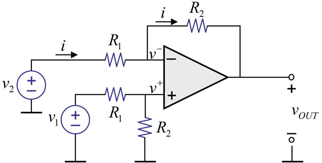
$$v^+ = v_1 \frac{R_2}{R_1 + R_2}$$
