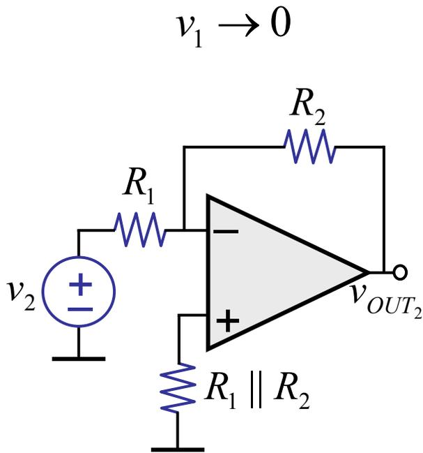
$$v_{OUT_2} = -\frac{R_2}{R_1} v_2$$
