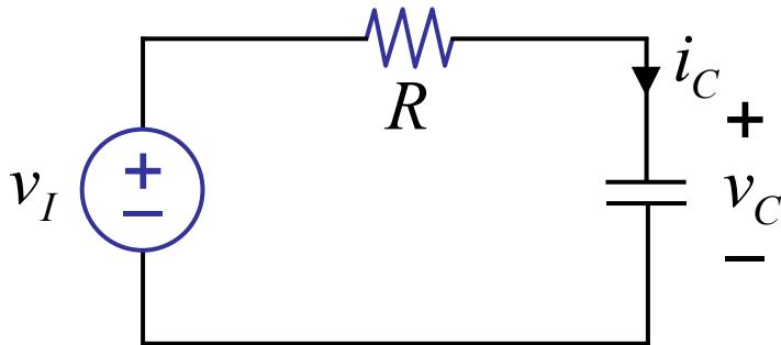
$$v_I(t) = \begin{cases} V_i \cos \omega t & \text{for } t \geq 0 \\ 0 & \text{for } t < 0 \end{cases} \quad (V_i \text{ real})$$
