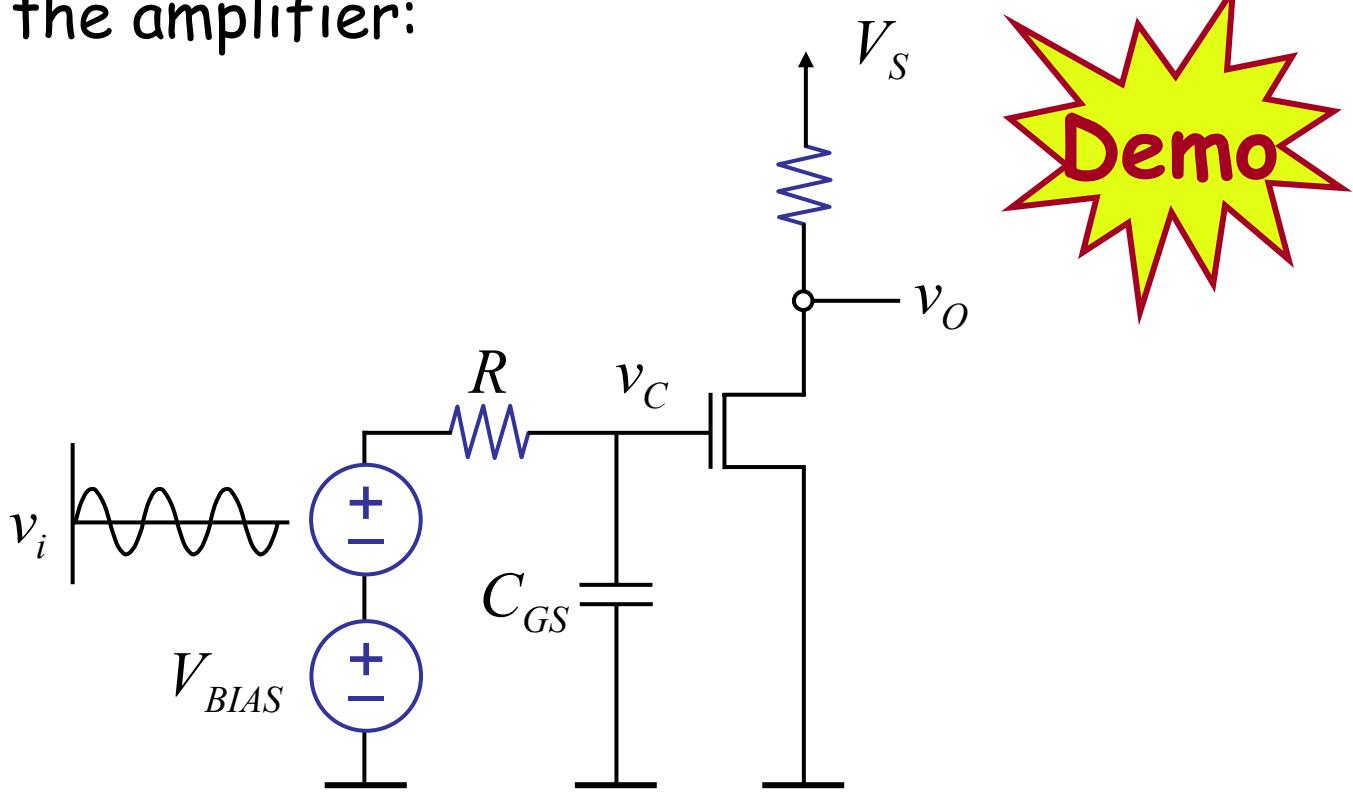
Observe  $v_o$  amplitude as the frequency of the input  $v_i$  changes. Notice it decreases with frequency.
