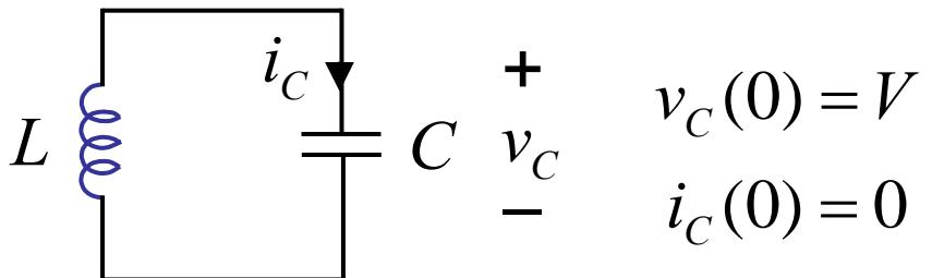
We can obtain the answer directly from the homogeneous solution ( $V_0 = 0$ ).
