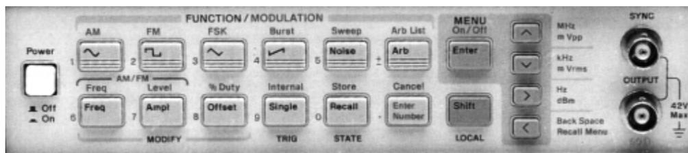
**Figure 6** The HP33120A Function Generator Control Panel
