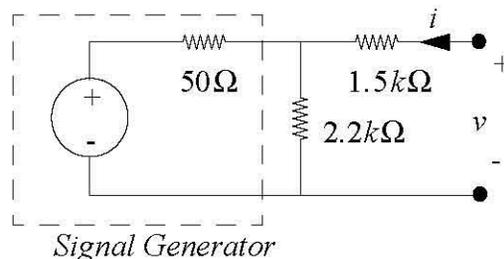
Figure 4: Experimental source-resistor network.
