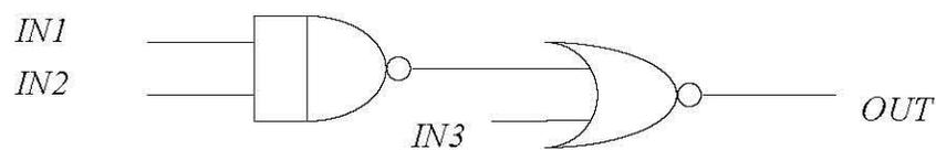
Figure 3: Combinational logic circuit for Pre-Lab Exercises 1-4 and 1-5.
