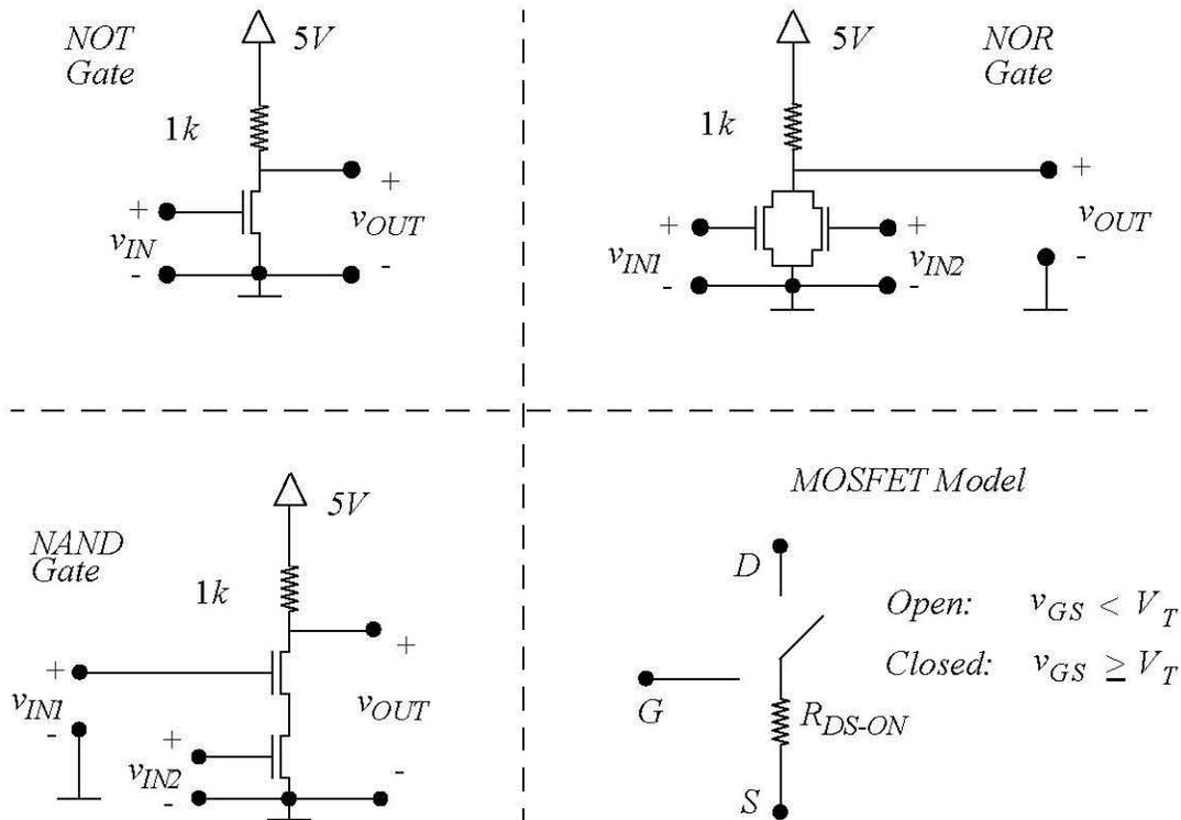
Figure 2: A NOT gate, a NOR gate, a NAND gate, and the switch-resistor MOSFET model.
