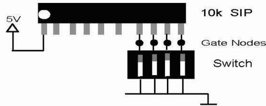
Figure 7: Switch pack and resistor array setup
