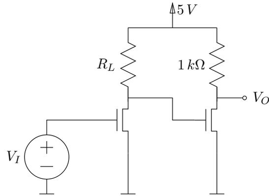
Given that  $V_I = 5\text{ V}$  and  $V_O = 5\text{ V}$ , and that the MOSFETs are accurately represented by the switch-resistor model, where the threshold voltage  $V_T = 2\text{ V}$  and the on-resistance  $R_{ON} = 100\ \Omega$ , find the minimum value of  $R_L$  which will allow this buffer to operate correctly.
