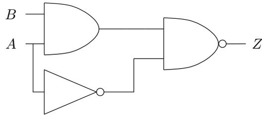
Fill in the truth table for the above digital circuit.
