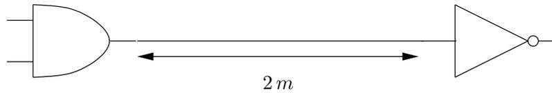
Noise in the 2 meter digital channel shown above is added in at the rate of  $0.6 V$  per meter. To correct for that noise, we introduce buffers into the channel. The purpose of a buffer is to take a signal, to which noise has been added so that it no longer meets the output specifications of the static discipline, and clean it up so that it once again meets the output specifications of the static discipline. These buffers, as well as the gates shown, obey the following static discipline:
