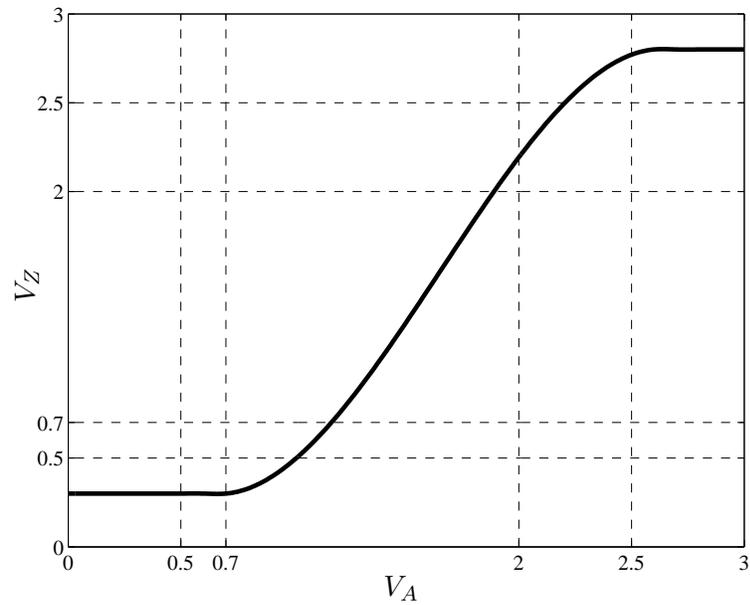
$$\begin{array}{ll} V_{OL} = 0.5 V & V_{OH} = 2.5 V \\ V_{IL} = 0.7 V & V_{IH} = 2.0 V \end{array}$$
