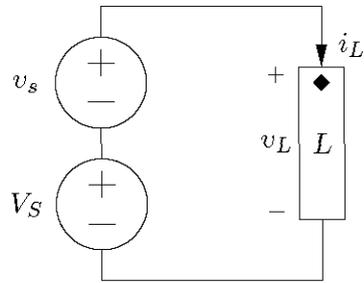
For the above circuit,  $i_L = 3v_L^3$ . If  $V_S = 1\text{ V}$  and  $v_s = 0.001 \sin(\omega t)$ , circle the correct expression for  $i_L$ .
