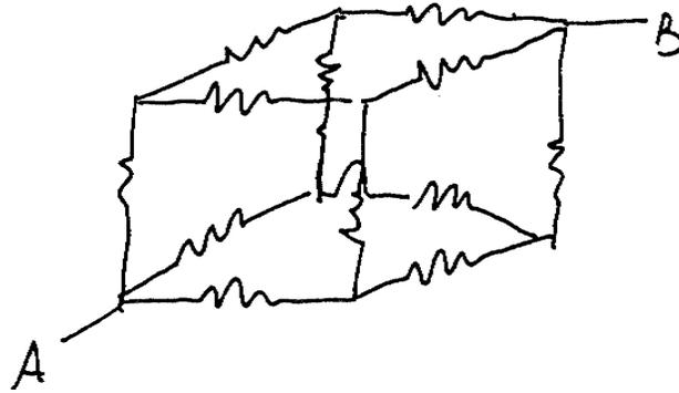
Calculate the equivalent resistance  $R_{eq}$  seen between the nodes  $A$  and  $B$  in the circuit shown above. Assume that all of the resistors have a value of  $1\Omega$ , and that 1 amp flows into node  $A$  and out of node  $B$ . (*Note: this problem can be solved without writing any node equations.*)
