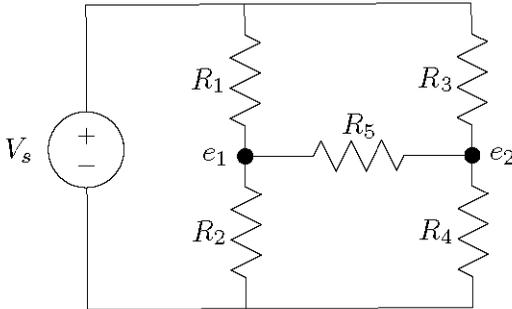
Write the node equations for the nodes  $e_1$  and  $e_2$  in the box below.
