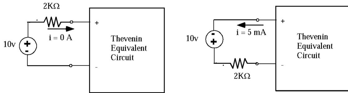
The current  $i$  is measured in two experiments which are performed on a Thevenin equivalent circuit as shown. What is the Thevenin equivalent resistance?
