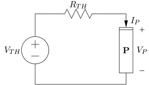
The device **P** in the circuits above is a nonlinear device. The circuit in the left-hand figure above that includes this device can be represented by the equivalent circuit which is illustrated in the right-hand figure. Find expressions for  $V_{TH}$  and  $R_{TH}$ .
