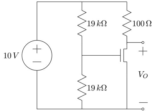
Find the power dissipated in  $R_{ON}$ , if the MOSFETs are accurately represented by the switch-resistor model, where the threshold voltage  $V_T = 2\text{ V}$  and the on-resistance  $R_{ON} = 100\ \Omega$ .
