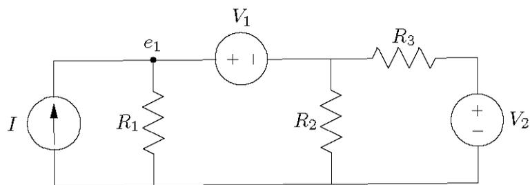
Following the node method, write a single node equation involving the node voltage  $e_1$  in terms of  $I, V_1, V_2, R_1, R_2$  and  $R_3$ .
