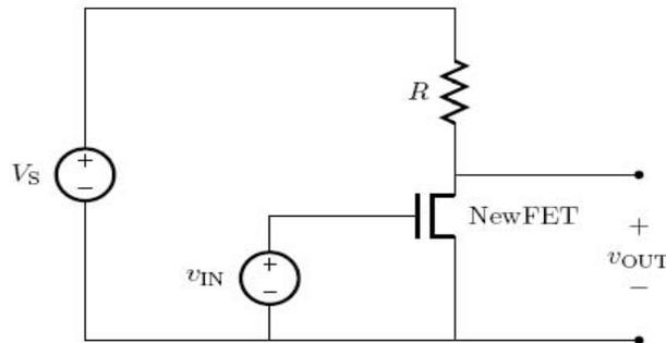
Figure 3: The NewFet used as an amplifier.
