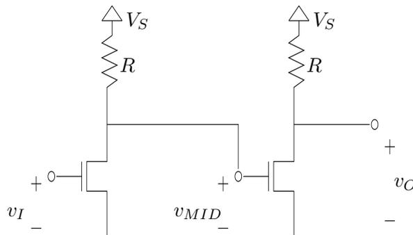
Figure 1: A two-stage non-inverting MOSFET amplifier is shown above. In this problem,  $V_I$  is chosen such that  $V_I = V_{MID} = V_O$
