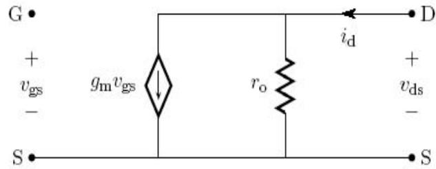
Figure 4: Small-signal model of the NewFET when biased in its active region.
