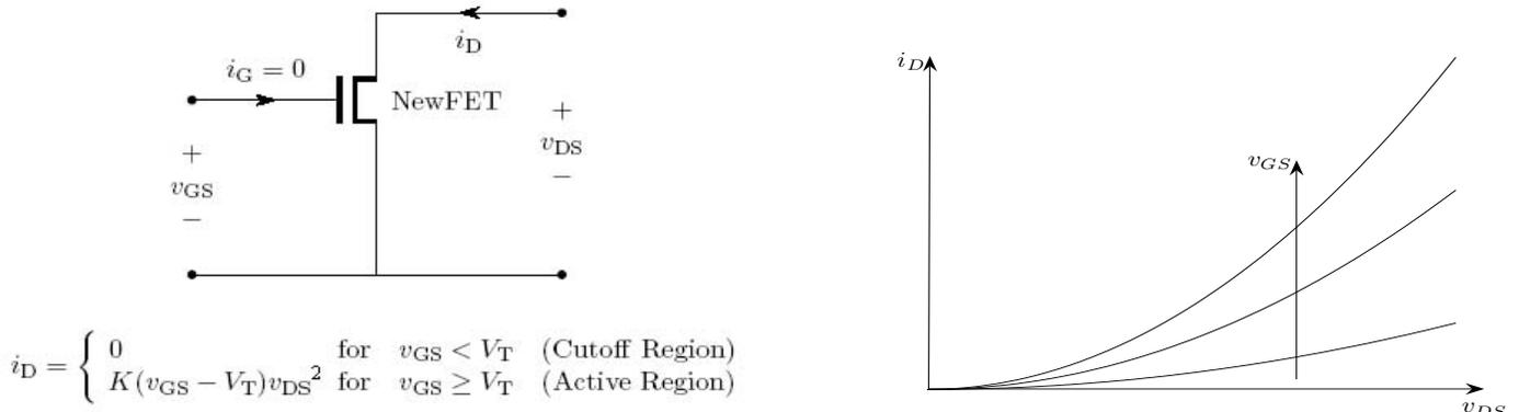
Figure 2: Large-signal characteristics of the NewFet.
