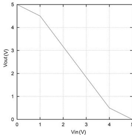
Figure 1: Input/Output transfer characteristic for inverter of Problem 3.2.
