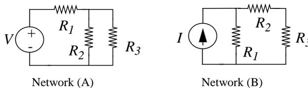
**Exercise 2.3:** Following the node method, develop a set of simultaneous equations for the network shown at the top of the following page that can be used to solve for the three unknown node voltages. Express these equations in the form
