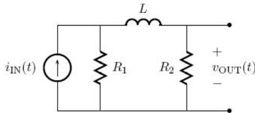
Figure 2: A first-order network driven in steady-state
