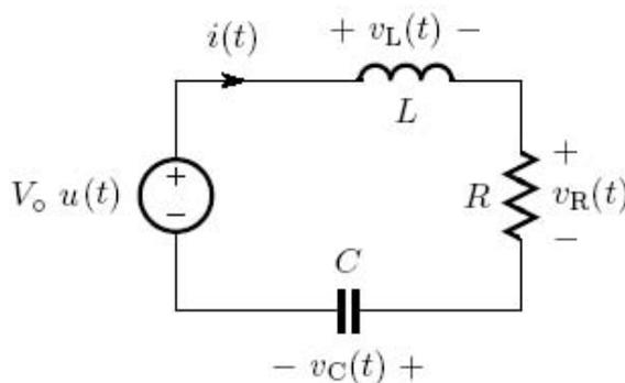
Figure 1: A step-driven series RLC circuit.
