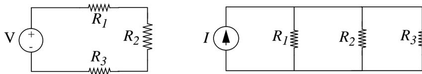
**Exercise 1-2:** Using only 1k resistors, synthesize a resistor of 3/5k and a resistor of 5/3k. Use no more than four 1k resistors in each case.
