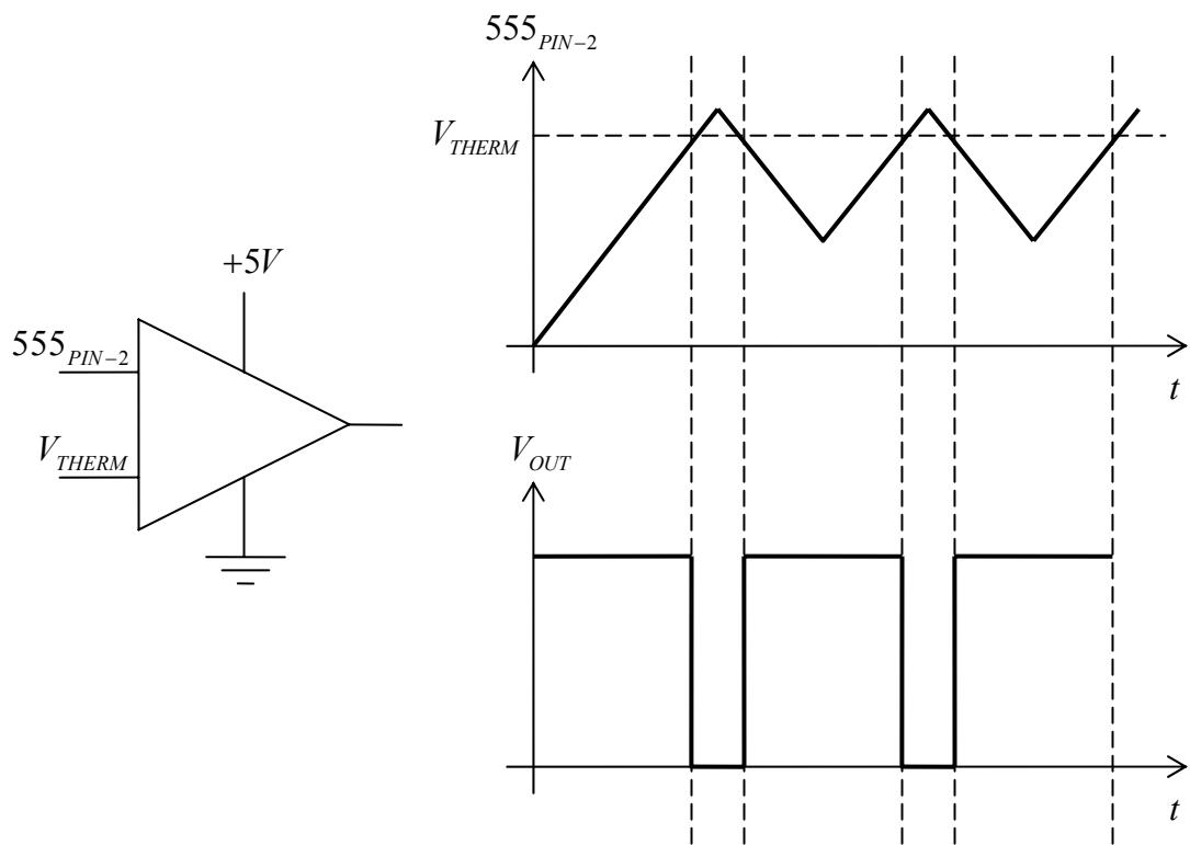
Since  $V_{THERM}$  is a variable voltage, use a comparator to control the average voltage delivered to the motor. If  $V_{THERM}$  increases (implying higher temperature), the output of the comparator will have a higher duty cycle and the motor will spin faster. If  $V_{THERM}$  decreases, the duty cycle of the output decreases and the motor spins slower.
